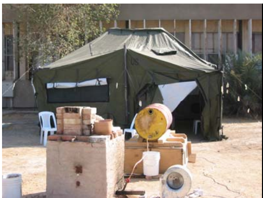
(Above left: brick kiln with diesel drum & air blower. Peep hole and temperature probe hole visible in kiln. Manifold had inlet for fuel and air and burns directly into kiln. Above right: setup inside kiln with fire box on bottom, pyrometric cone, and circular pedestal for the pot. Kiln was lined with fiberfax heat insulative blanket.
