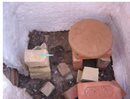
(Above left: brick kiln with diesel drum & air blower. Peep hole and temperature probe hole visible in kiln. Manifold had inlet for fuel and air and burns directly into kiln. Above right: setup inside kiln with fire box on bottom, pyrometric cone, and circular pedestal for the pot. Kiln was lined with fiberfax heat insulative blanket.
