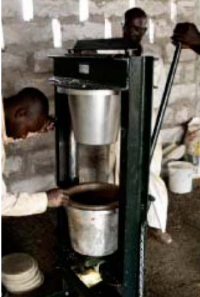
Figure 2 Filter Press (from www.potpaz.com )
